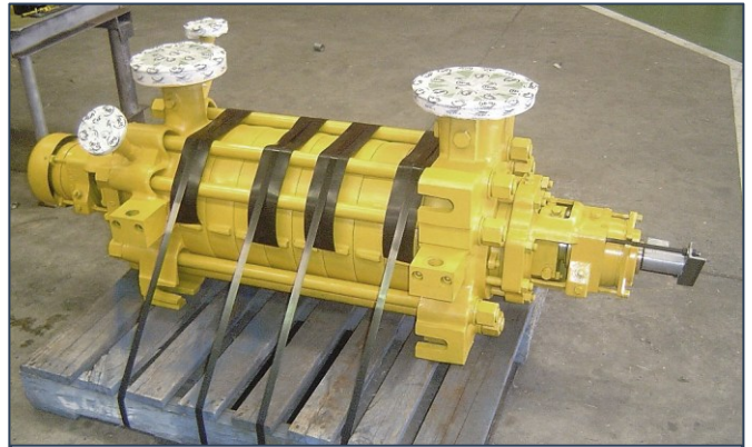
Overhaul of boiler feed pump at the workshop
